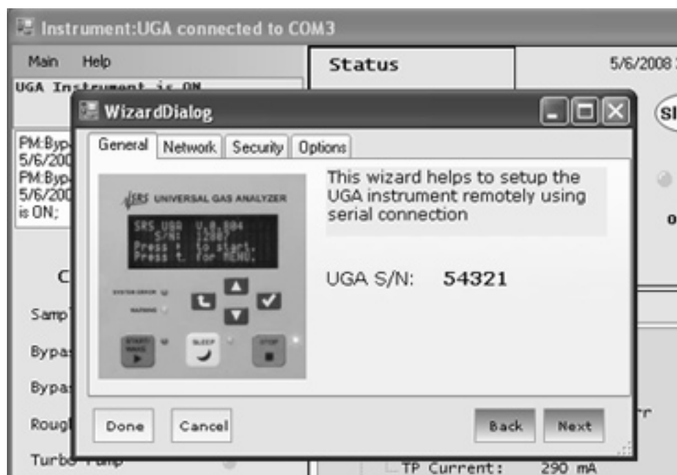
Fig. 2-7. Screenshot of the 'Wizard' dialog box in the 'Main' menu of UGA control software.
